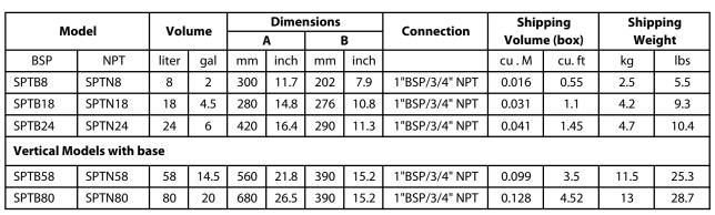
All connections are stainless steel unless stated otherwise. Tank precharge: 15psi / 1 bar
